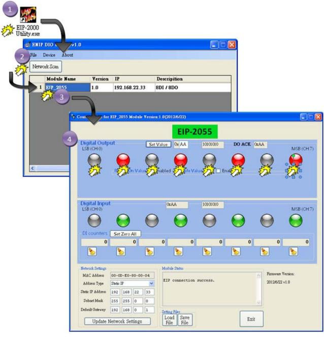
Figure 3-3. the steps to test EIP-2000 Utility
