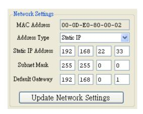
The <u>Address Type</u>, <u>Static IP Address</u>, <u>Subnet Mask</u> and <u>Default Gateway</u> items are the most important network configuration and should always match the LAN definition of your PC. Or, the connection between the EIP-2000 and your PC may have problem. Contact your network administrator to obtain a proper network configuration for the EIP-2000.
