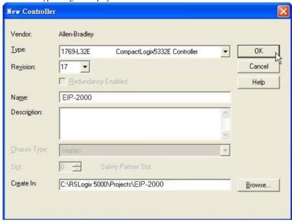
Figure 7-2. Set the PLC type and project name.
