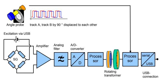
Block diagram for sensor with integrated electronics.
