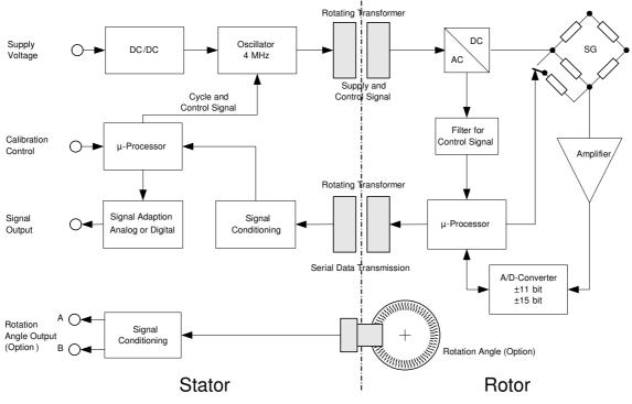
Block diagram for serial signal transmission
