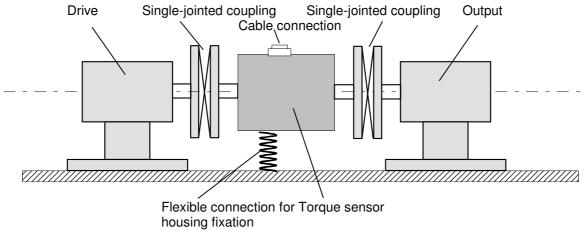
In this case, with both single-jointed couplings, the torque sensor forms a double-jointed coupling. A single-jointed coupling can only balance axial and angular misalignments.
