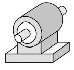
Shafts have to be cleaned with solvent (e.g. acetone) before the assembly No foreign bodies may adhere to them.
