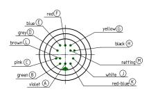
View: socket on soldering side
