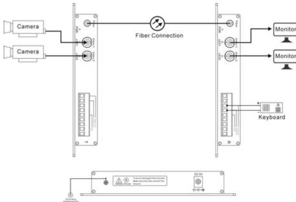
To install, connect the video inputs to the SWV60201-T, connect the video monitors or other video receptors to the SWV60201-R, and connect an appropriate optical fiber between the SWV60201-T and SWV60201-R optical ports. Connect data signal sources or destinations, as required, to the "DATA" port per the following Built-In Data Connection section.
